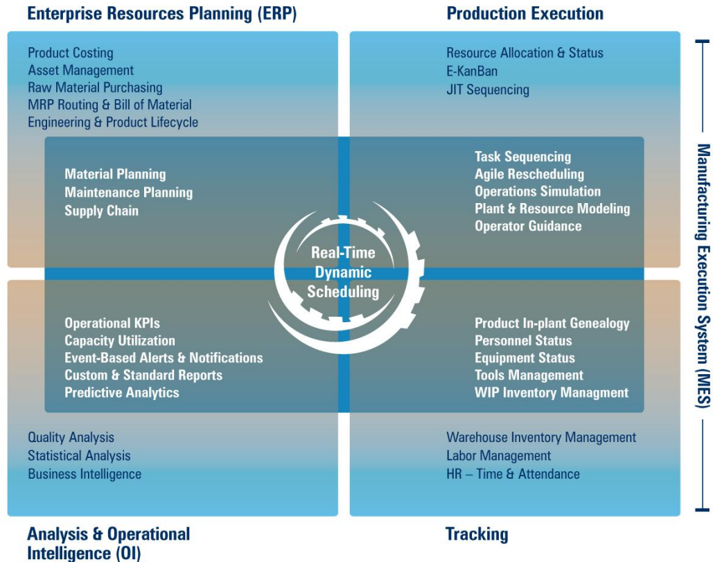
Figure 3: The new category of software combines the factory-driving pieces of the four functional areas with a dynamic scheduling engine at the core to cope with constant change.
